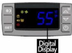
The temperature displayed on the control indicates the real-time air temperature as measured by Probe 1 (P1) located behind the front grill of the cooling unit.
