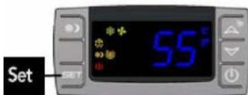
The cooling unit is factory preset with a Minimum Set Point of 58°F and a Temperature Differential of 4°.
