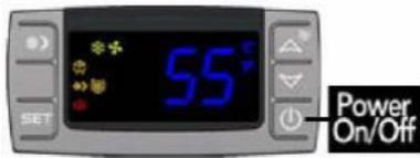
Press "Power" to turn the unit on and off.
